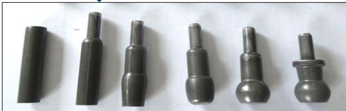
Real Forging Process
